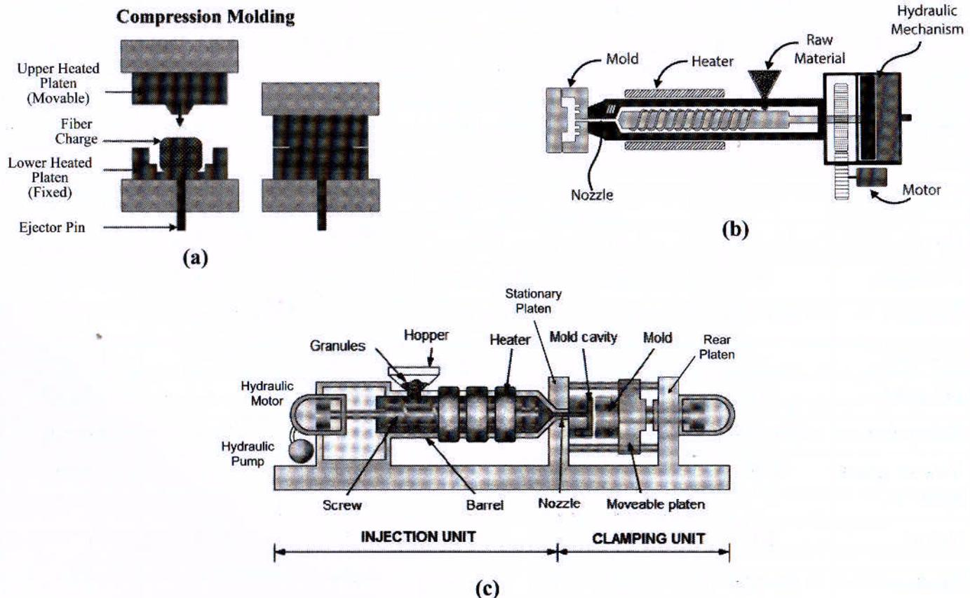
**Figure 3. (a) Compression, (b) extrusion and (c) injection molding machines**
